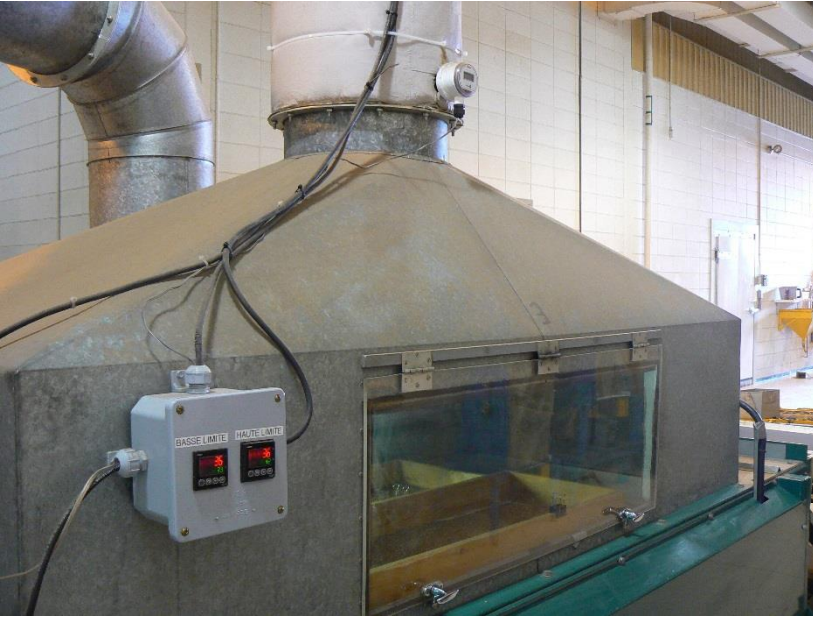
Water activity integrated into BCC drying line at the Berthier Tree Seed Centre
