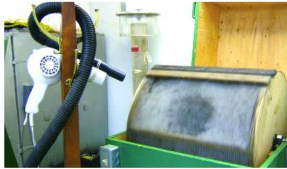
Figure 3. Catkins being processed in a cone tumbler with a screen wrap with air flow provided by a combination of a shop vacuum and hair dryer. Photo by Bernard Daigle
